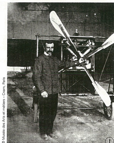
Blériot VIII à hélice quadripale, 1908. The Blériot VIII with its four-bladed propeller in 1908.
